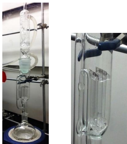
Figure 3.1 Photograph of PDMS substrates undergoing Soxhlet extraction in ethanol.
