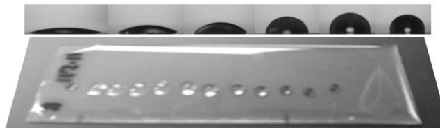
Figure 4.4 Photograph of spreading water droplet profiles along PDMS surface gradient. The spreading of water drops on PDMS and glass surface gradients indicate the variation of the SAM chemistry induced by spatiotemporal UVO exposure.
